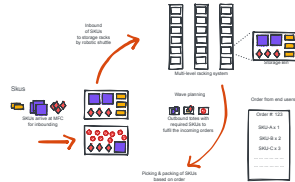
Flow of inbound and outbound in a fulfilment centre in which multiple store keeping units (SKUs) are allocated to the same storage bin.
